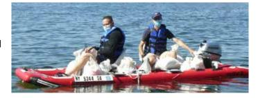
The FastCat12 has four floatation chambers; two side chambers and two floor chambers. The boat will stay afloat and can be paddled or motored when loaded to capacity with the main chamber deflated.
